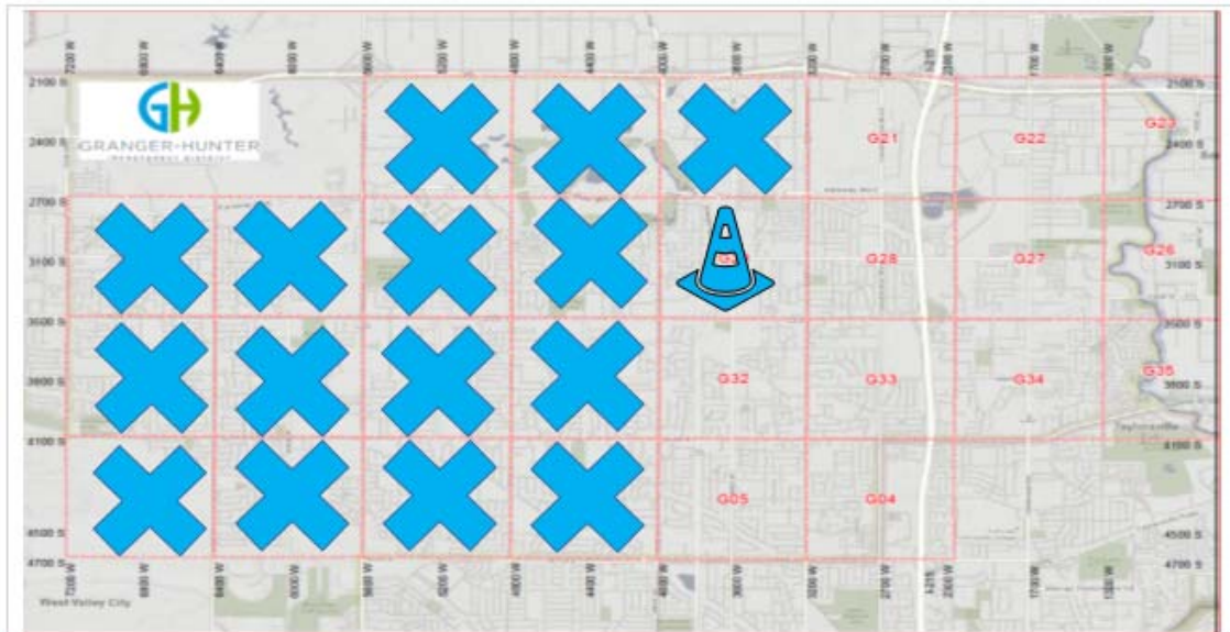
Figure 10: Current 2019 map of the fire hydrant inspections, the “X” indicates the area is complete and the cone indicates the current location of inspections taking place.
